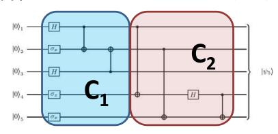
**Proof:** Savitch's Theorem! Recursively divide C into two chunks,  $C_1$  and  $C_2$ , with d/2 layers each. Then
